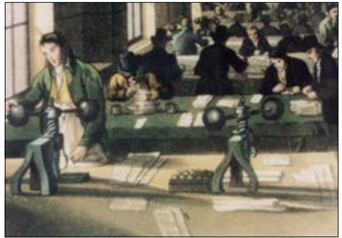
Detail from “The Stamp Office at Somerset House” -- an employee operating a hand operated Screw Press. An aquatint from Rudolph Ackermann's “Microcosm of London” 1809.
