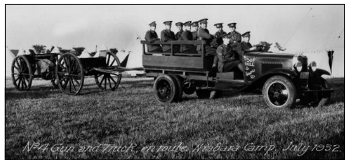
This picture is indicative of the ill-equipped state of Canada's militia. The sole concession to modernization for the artillery was to replace the wagon wheels on the 18-pounder gun and its ammunition trailer with inflated, rubber wheels in 1933-34. Courtesy of Jim Smith of Niagara-on-the-Lake.
