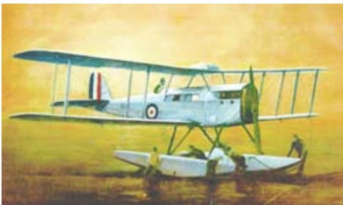
**Pictured is the RAAF De Havilland DH50A floatplane serialled A8-1, which flew to the Pacific Islands in 1926. The pilot sat in the cockpit while the other two crew members were accommodated in a small cabin ahead of the cockpit. Artwork by Peter Connor.**
