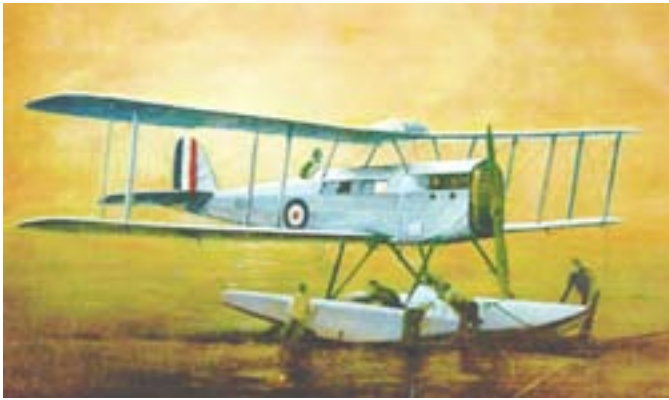
Pictured is the RAAF De Havilland DH50A floatplane serialised A8-1, which flew to the Pacific Islands in 1926. The pilot sat in the cockpit while the other two crew members were accommodated in a small cabin ahead of the cockpit. Artwork by Peter Connor.
