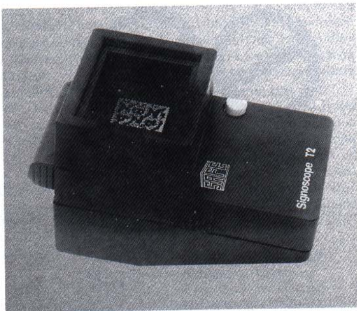
The SAFE Signoscope T2 watermark detector is one of the electronic models currently available. Although relatively expensive, it eliminates all danger of exposure to chemicals or damage to stamps.
