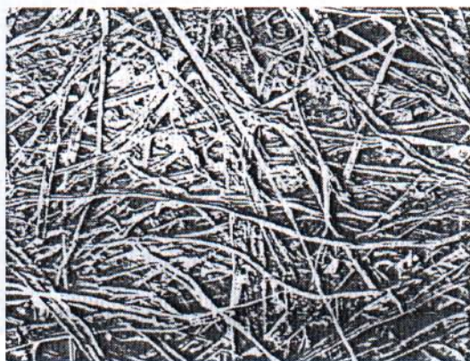
Eraser residue from a Magic-Rub block eraser, magnified 100 times. Residue and fibre damage are relatively low.
