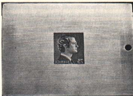
(A) The Die - After tempering in an 800 C bath of sodium cyanide for 25 to 30 minutes, the red hot plate is removed and quickly hardened by immersing in cold water making the steel very hard.
