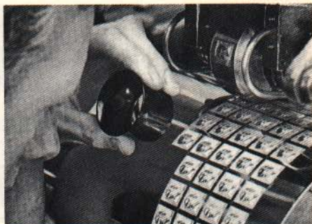
(D) After tempering the transfer roller is put in a machine which imprints the printing cylinder. The cylinder is steel with a thin layer of copper.
