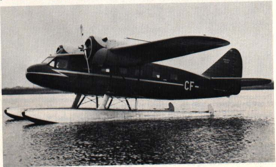
Fairchild 45-80 Sekani on EDO floats. Photo: Museum of Science and Technology, Aviation and Space Section, Ottawa.
