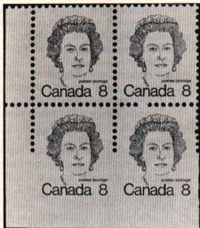
Figure 3. 1973 8c QE II Caricature definitive (CBN printing) partly imperforate due to missing strike of the perforator (photo by Wayne Cuddington).
